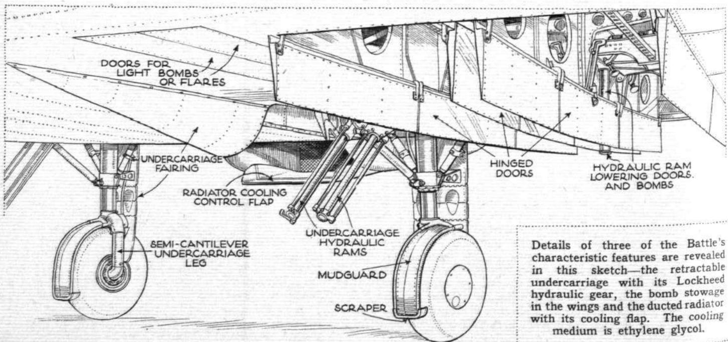
Details of three of the Battle's characteristic features are revealed in this sketch—the retractable undercarriage with its Lockheed hydraulic gear, the bomb stowage in the wings and the ducted radiator with its cooling flap. The cooling medium is ethylene glycol.
