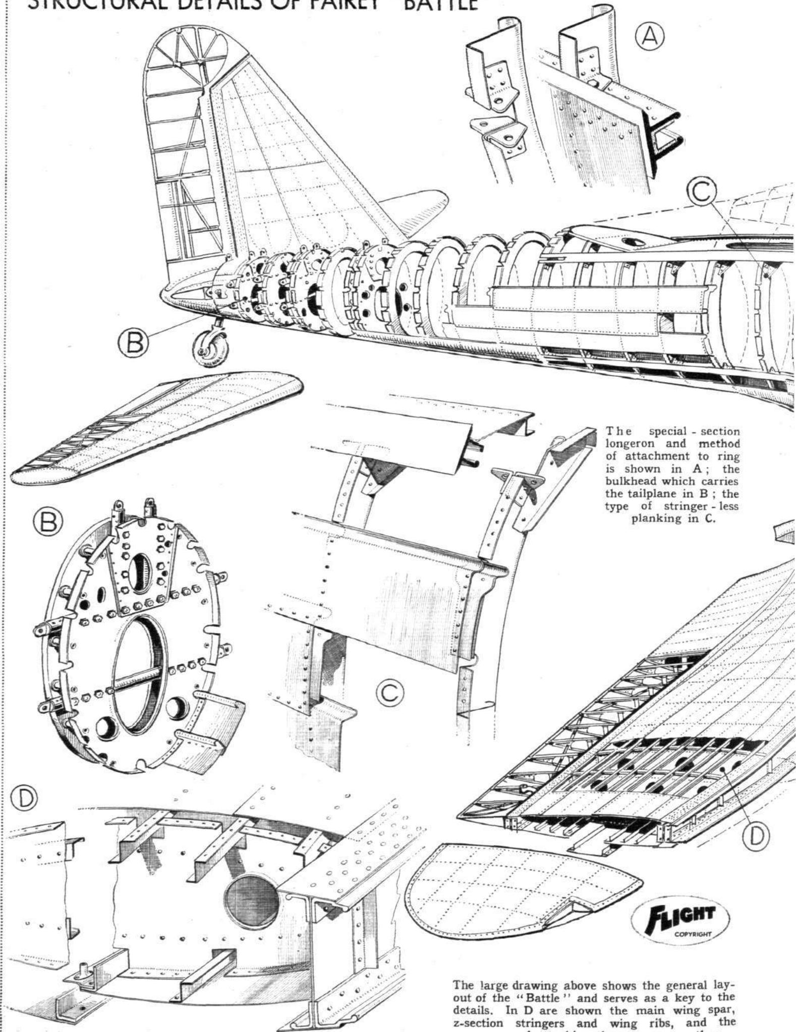
The special-section longeron and method of attachment to ring is shown in A; the bulkhead which carries the tailplane in B; the type of stringer-less planking in C.
