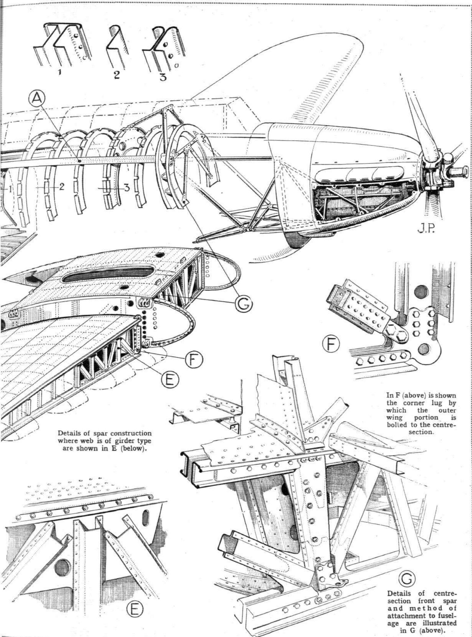
Details of spar construction where web is of girder type are shown in E (below).
