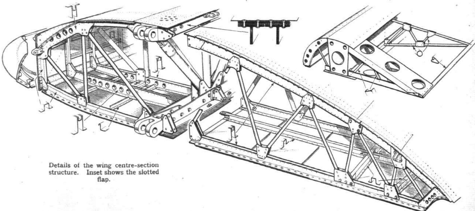
Details of the wing centre-section structure. Inset shows the slotted flap.
