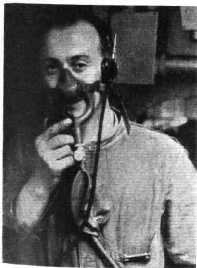
The oxygen mask as used by the crew of the Consolidated 28-5 leaves the mouth free to use the intercommunication system which extends throughout the boat.
