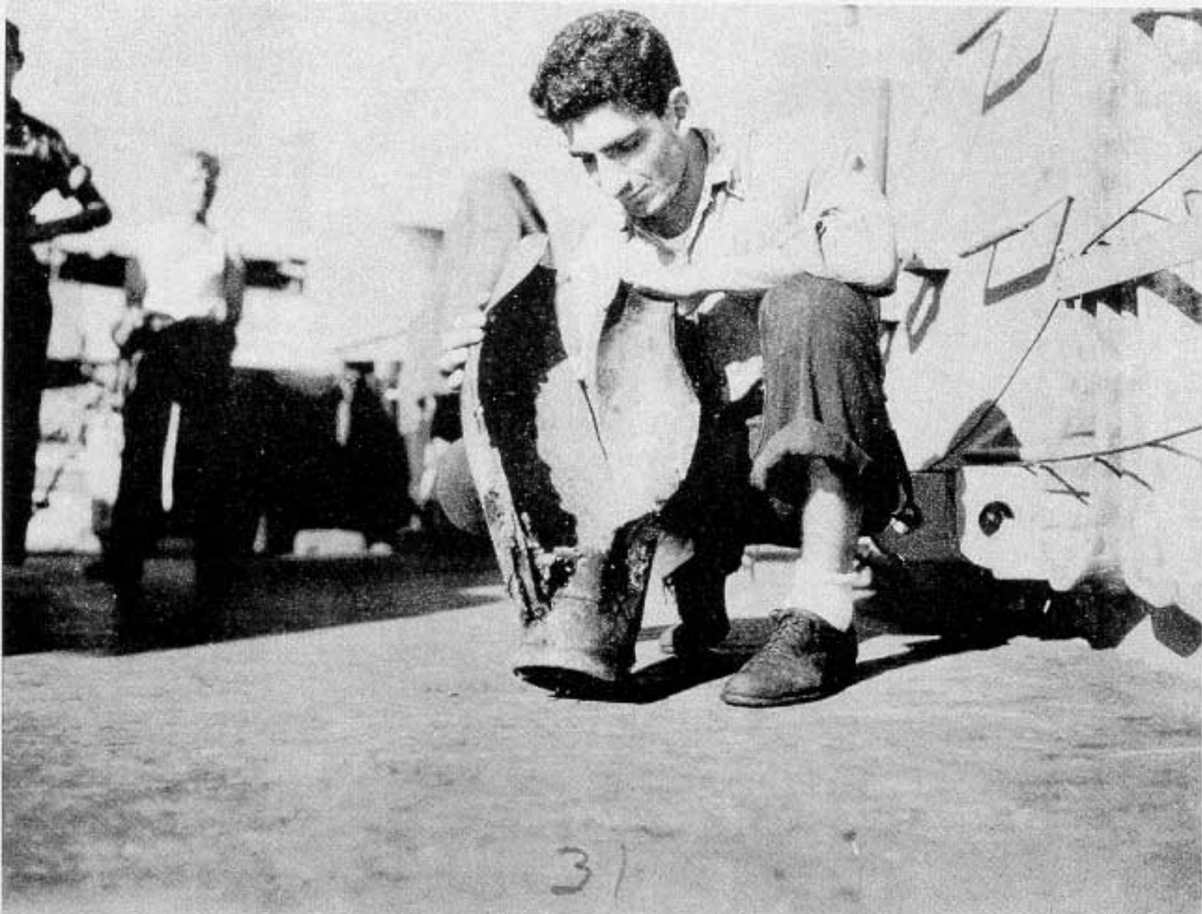
Photo 31: One of two 6-inch/47 H.C. projectiles — that detonated in the gun room of No. 3 turret. Both are believed to have been stowed in the left projectile rack, 30 inches below the roof. Both went off 24 minutes after the bomb hit, during which time there was a fire in the gun room. Detonations were apparently low order. The left side plate of the turret was bulged outward in way of the stowage to a depth of 4 inches.
