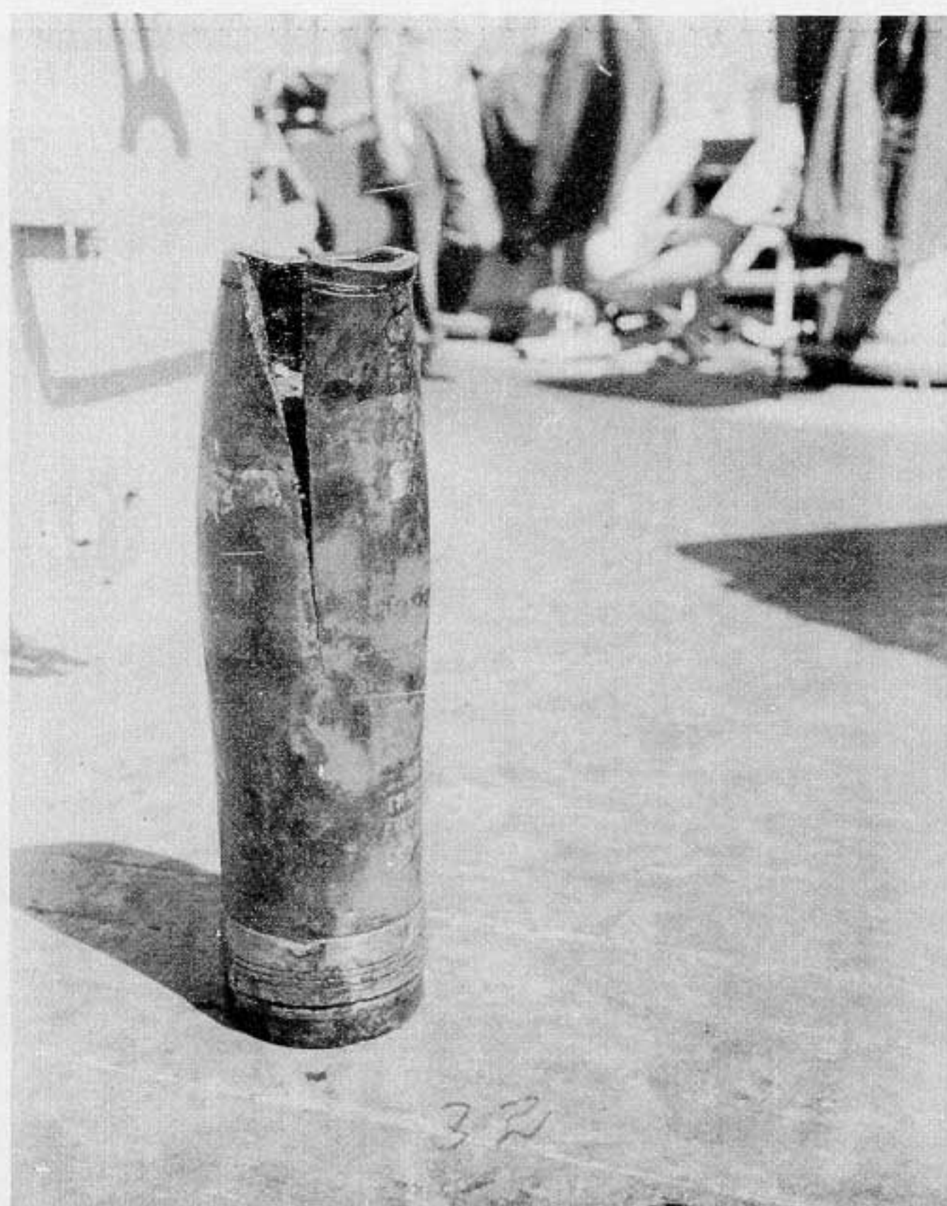
Photo 32: A 6-inch/47 H.C. projectile split open by impact. The filler did not detonate or burn. Recovered from the gun room of No. 3 turret.
